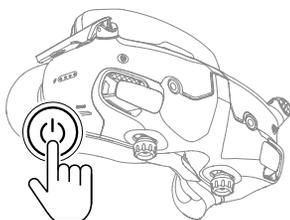
Press the power button once to check the current battery level.
