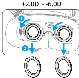
2. Take out the -2.0D Corrective Lenses and peel off the protective film. Distinguish the left and right lenses via the L and R marks on the bottom.
