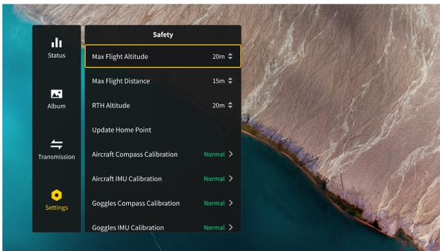
To exit or return to the previous menu, push the accelerator forward, or gently press the accelerator when the cursor is on any empty spot on the screen.
