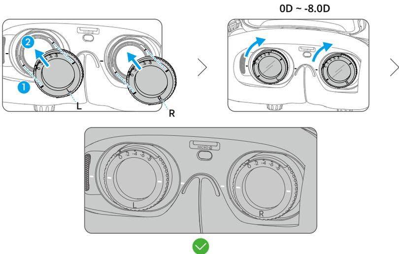
4. Adjust the diopters of the goggles according to your needs and lock the knobs.
