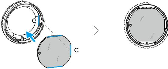
5. Make sure the lens is installed in the correct way and not tilted. Clean the lens with the lens cleaning cloth to wipe off fingerprints and dust.
