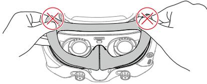
2. Align the positioning columns of the new foam padding with the positioning holes on the goggles. Install it and press along the contour. You will hear a "click" sound when pressing the two sides of the foam padding, check and make sure that there is no gap between the foam padding and the goggles.
